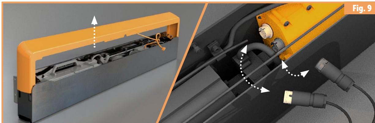
**Slide the top cover upwards and disconnect the solar panel (beige) and LED panel (dark grey) connectors from the control unit.** CAUTION! – Be sure to pull at the connector, not by the cable. Otherwise this may damage the cable. Put the cover and the battery in a safe place to prevent damage during subsequent handling.
